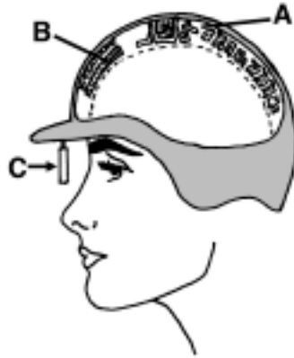
Figure C.9. Nanotechnology application: helmet incorporating P50 midlatency auditory evoked potential recording and near-infrared detection of frontal lobe blood flow to measure sensory gating and hypofrontality, respectively. A. Evoked potential module including audio stimulator (earphones), surface electrodes (vertex, mastoids, forehead), amplifiers, averager with wave recognition software, and data storage device for downloading. B. Near-infrared detection module for frontal lobe blood flow measurement. C. Flip-down screen for tracking eye movements and display of results from sensory gating and frontal blood flow measurements.
